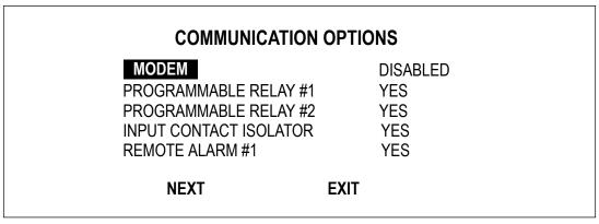
The Internal Modem Option allows the system to dial out or receive incoming calls. To set dialing features, and to enable internal or external modem, press MODEM on the first page of the Communications Options screen. The Auto Dial screen will be displayed.
